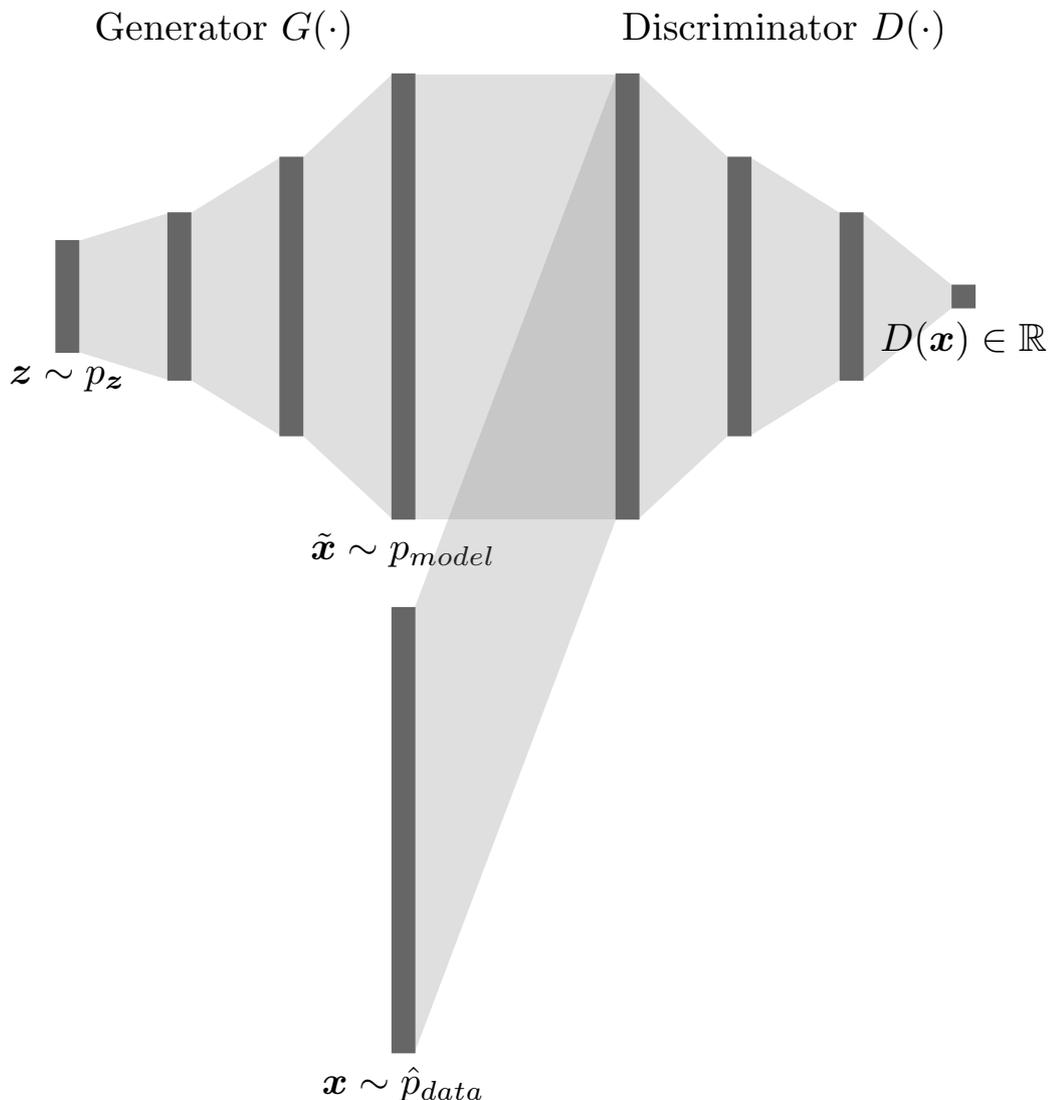
Figure 1.2: Illustration of GAN. The darker grey rectangles represent arrays of neurons and the lighter grey shapes are connections between them.
