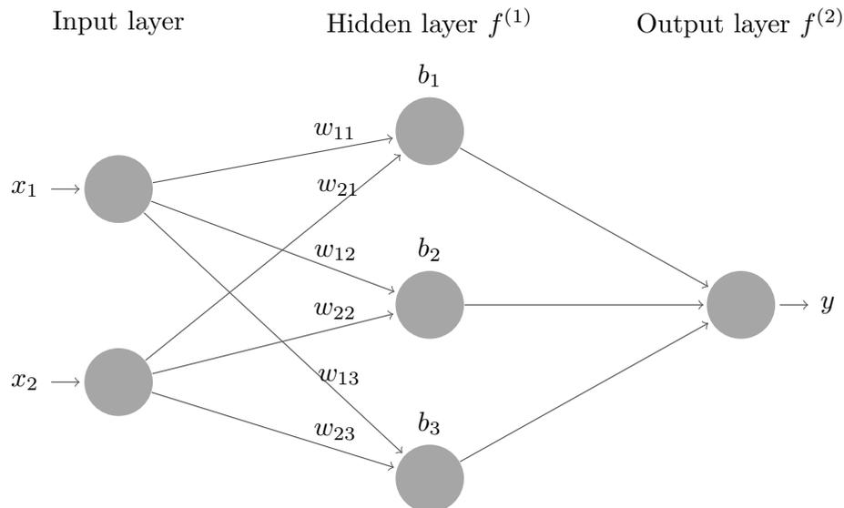
Figure 1.1: Neural network with input layer of size 2, one hidden layer of size 3 and output layer of size 1.
