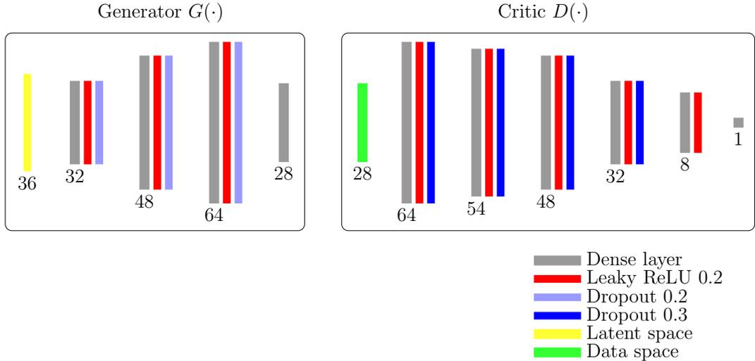
Figure 4.2: Diagram of our model. The numbers under dense layers denote their output sizes. The numbers under latent and data space denote the dimensionality.
